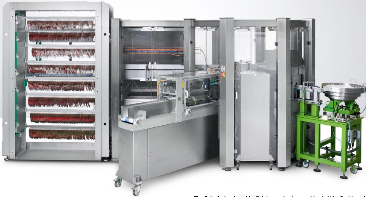
The Octo-1, developed by Belgian packaging machine builder Scaldopack, is a system for the production of stand-up pouch packs.
