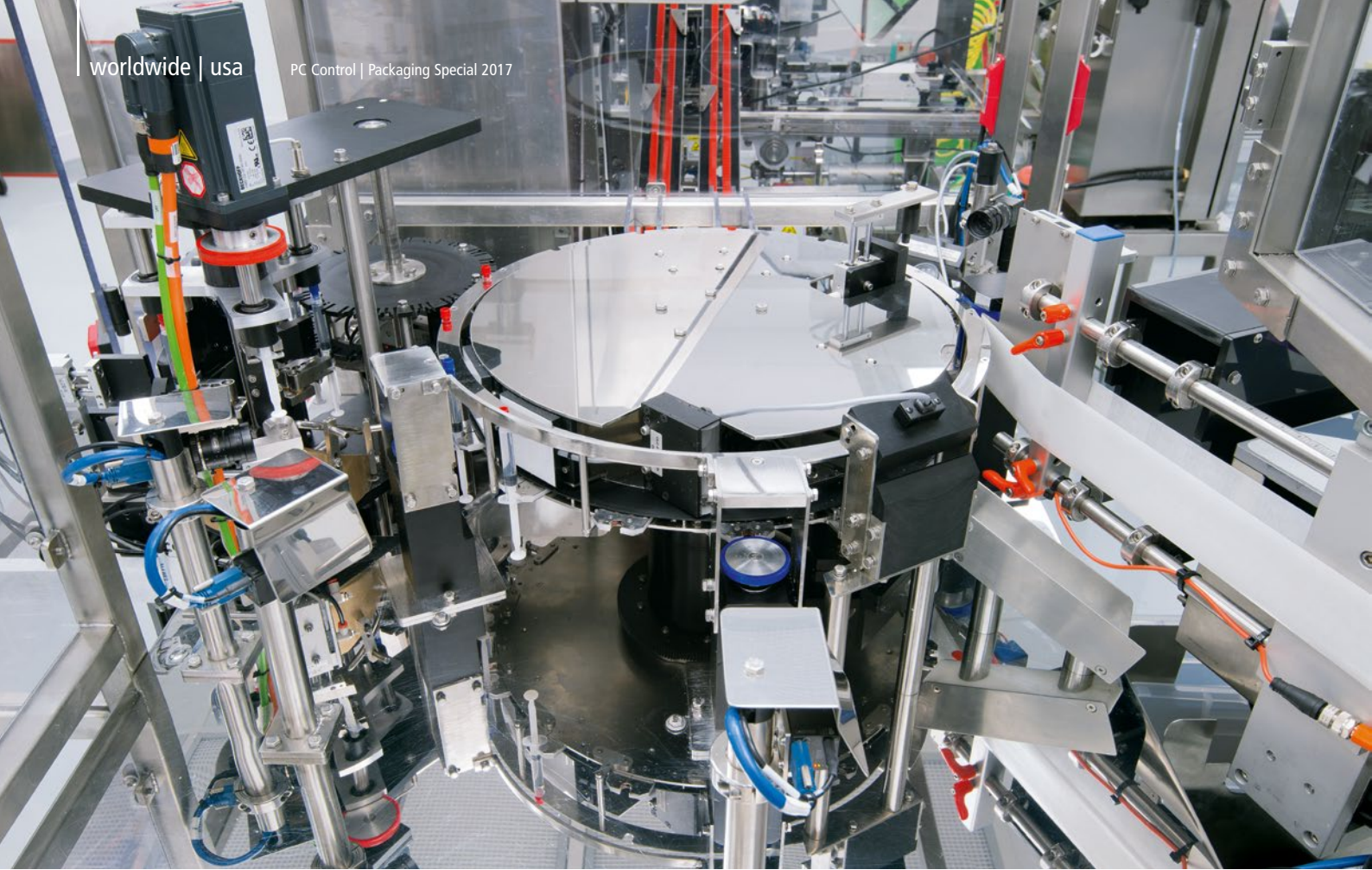
The SASI-30 inspection machine feeds syringes or vials through up to seven camera stations to assure that products adhere to stringent medical hygiene standards.
