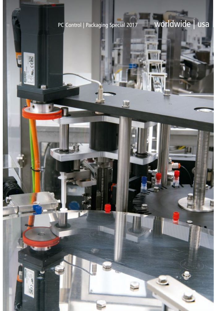
The servomotors of the AM30xx and AM81xx series provide robust, highly-accurate motion control.
