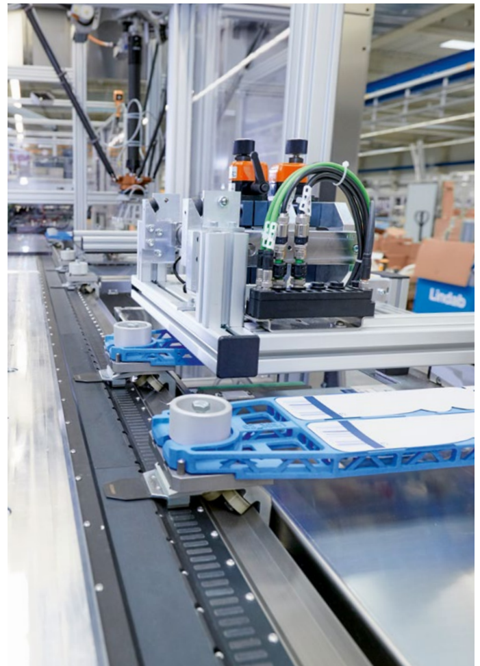
In the toothbrush packaging line developed by Koch Pac-Systeme (see p. 14) XTS replaces expensive mechanical systems with software functionalities that make the line more compact and more flexible for extremely fast product changeovers.
