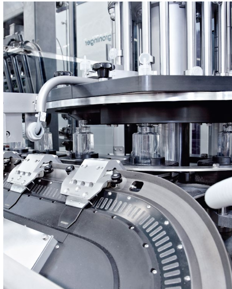
PC-based control is particularly innovative in combination with the eXtended Transport System (XTS), which combines high filling speed with extremely compact machine design in the Groninger cosmetics filling machine shown here.
