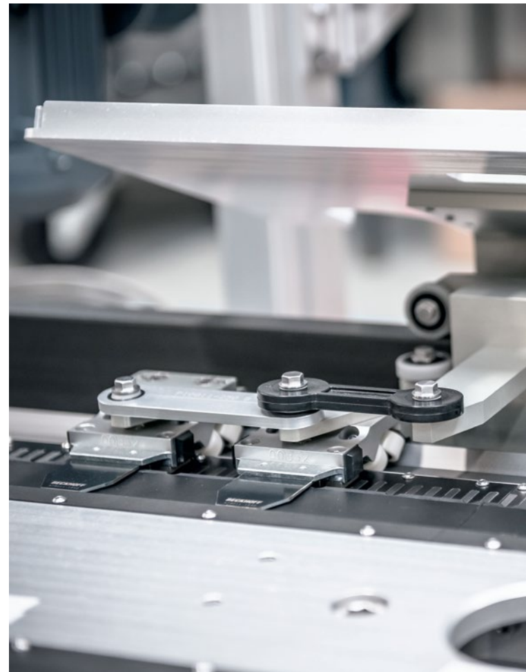
Graniten Engineering (see p. 22) decided to connect the XTS movers in pairs to ensure dynamic and precise transport of high payloads.
