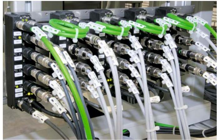
The I/O data points are acquired for the most part via EtherCAT Box Modules with IP 67 protection for a space-saving and flexible architecture as well as for a minimization in the number of switchboxes.
