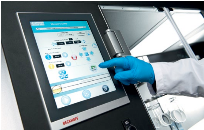
The machine is operated and controlled via a CP2912 multi-touch panel.
