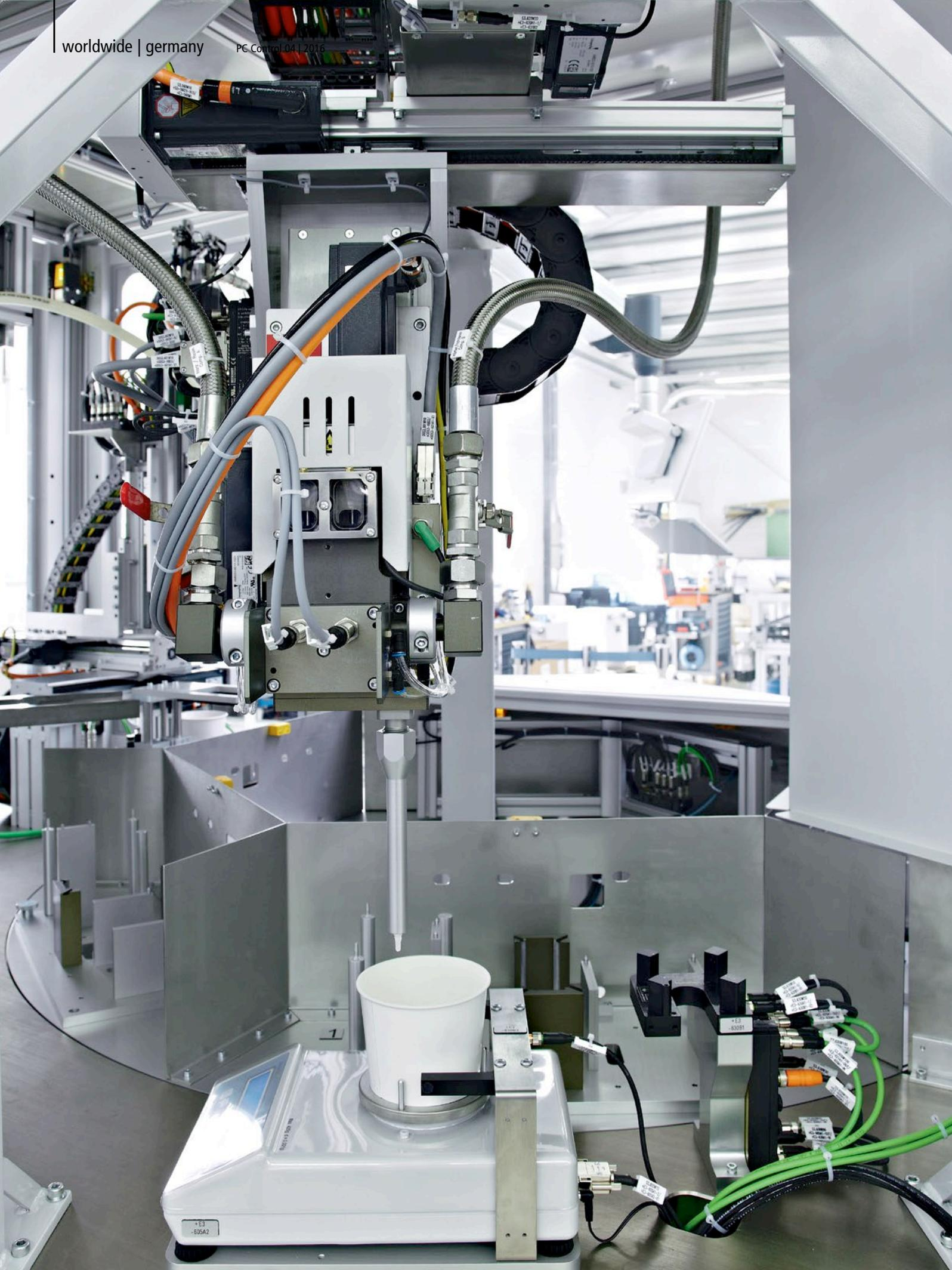
Fast, powerful, open: TwinCAT CNC automates dispensing system used in the automotive industry
