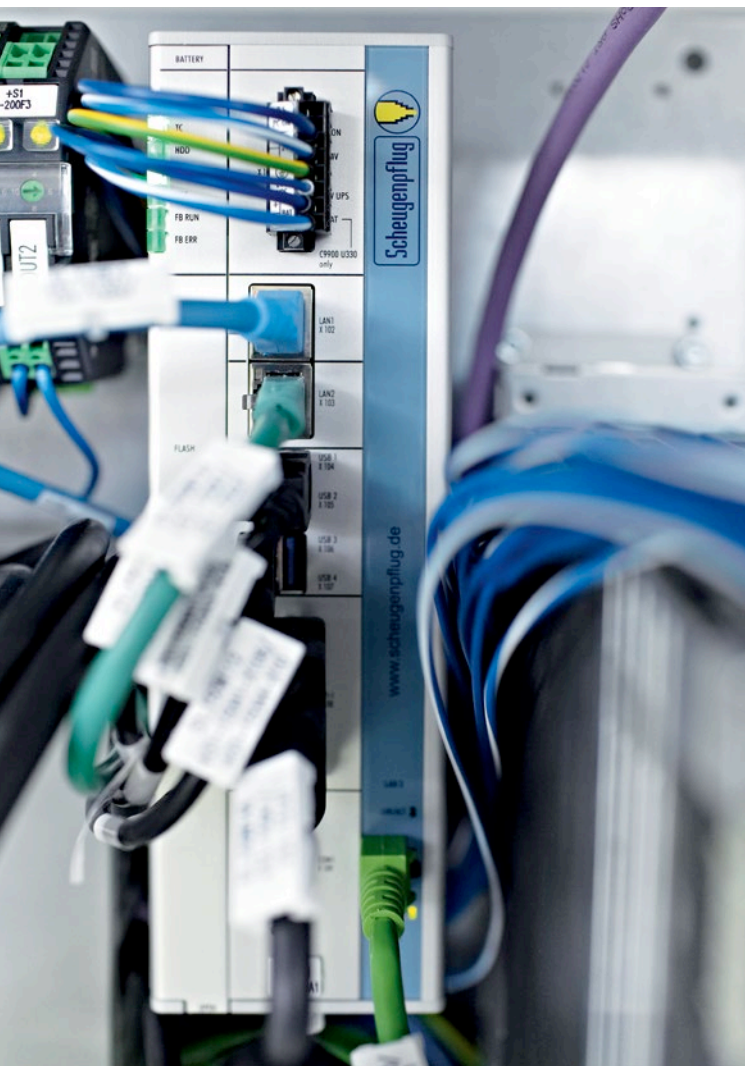
The C6920 Industrial PC from Beckhoff – seen here as a custom version with customer logo – controls the entire dispensing machine.
