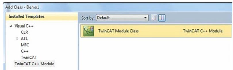
In addition to I/O configuration and PLC programming, C/C++ code can also be created in the TwinCAT 3 project. Wizards for the creation of basic projects, classes and I/O variables make efficient engineering possible.
