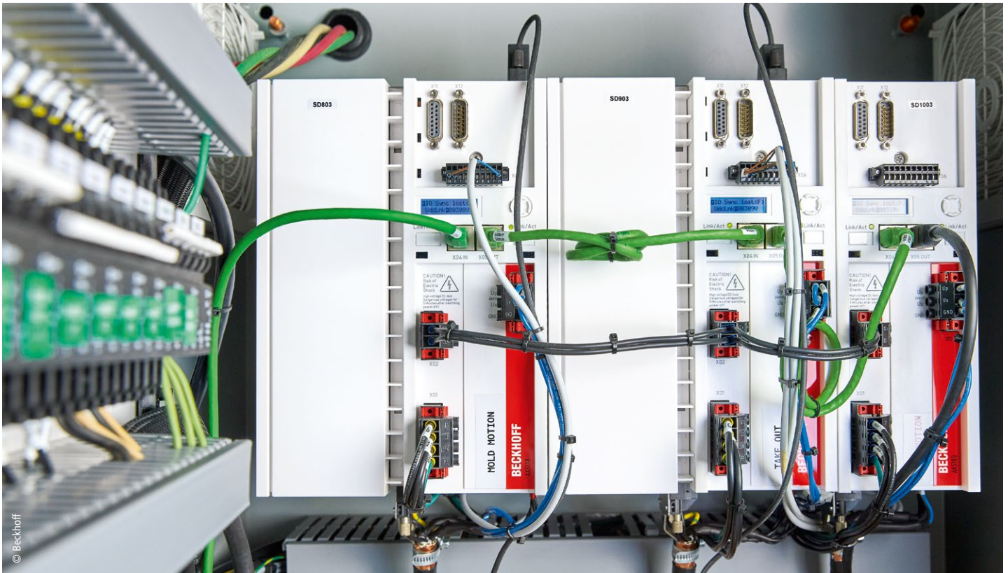
AX5000 series Servo Drives from Beckhoff provide dynamic motion control for the screw, linear mold movement and side-entry robot.
