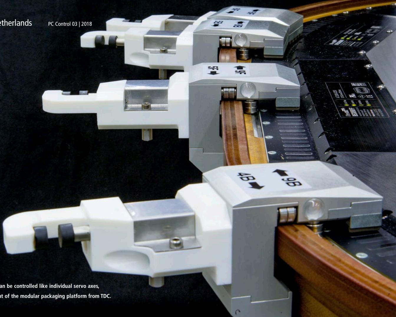
With its movers that can be controlled like individual servo axes, XTS is the core element of the modular packaging platform from TDC.
