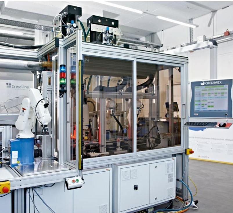
XTS links five process stations in this CresaLine version
