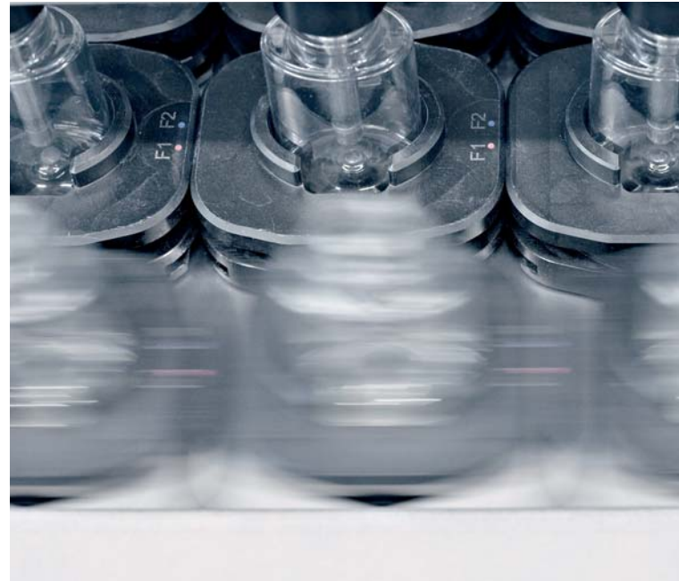
After filling, the batch of 10 bottles is accelerated from standstill and dynamically synchronized with the continuous sealing process.
