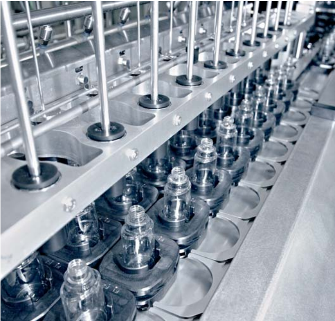
Batches of 10 bottles are filled with fragrance and then pushed into the gripping elements of the waiting XTS movers, together with their workpiece carriers.
