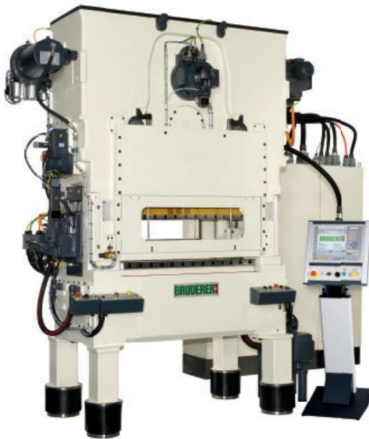
Swiss punch press manufacturer Bruderer has relied on Beckhoff PC-based control technology since 1998. The picture shows a high-speed BSTA 150 punch press.
