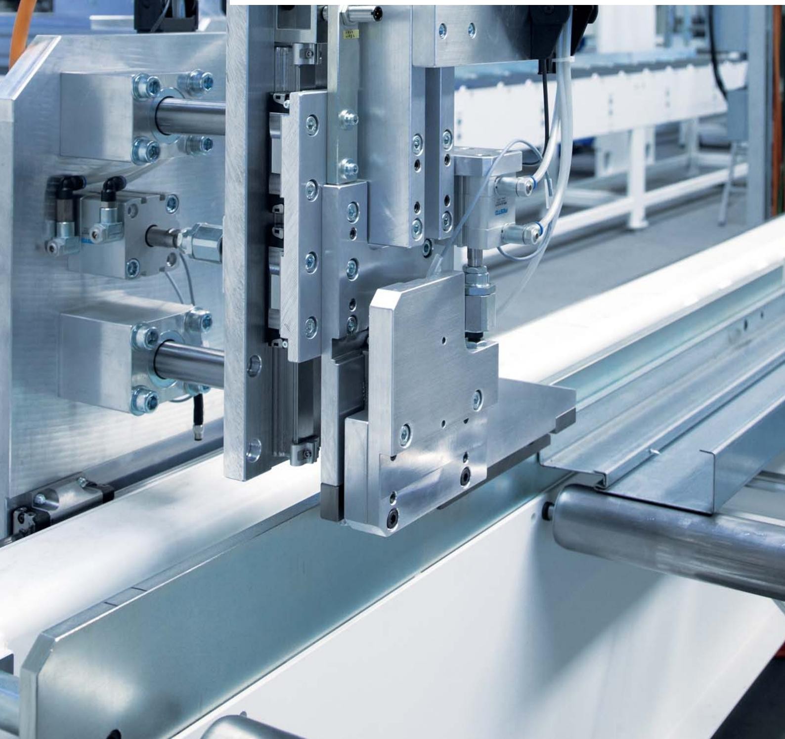
A door frame consists of two side jambs and a header. All three elements are made from beveled sheet metal and are mitered. The steel frame processing line for Hörmann consists of four saws, two gantries for material loading and several roller tracks for material handling. In addition to the saw unit the line also includes a laser cell with a special material supply concept and was extended with a complex punching machine during the course of the project.
