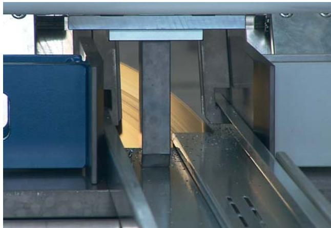
Based on an ERP order, all cutting and clamping parameters for the frame are calculated from the geometric dimensions at the saw inlet, so that the saw feed control is optimized at all times.
