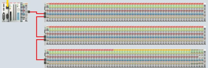
Each CX1000 controls around 180 Beckhoff Bus Terminals, which in turn deal with lighting, heating and ventilation control.
