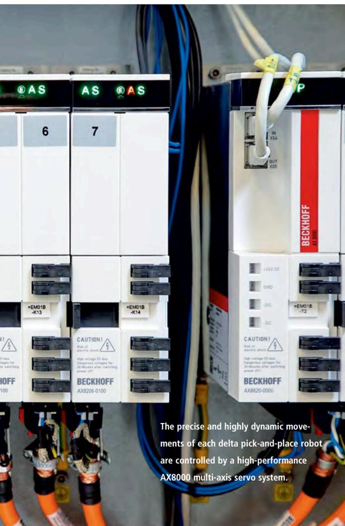
The precise and highly dynamic movements of each delta pick-and-place robot are controlled by a high-performance AX8000 multi-axis servo system.
