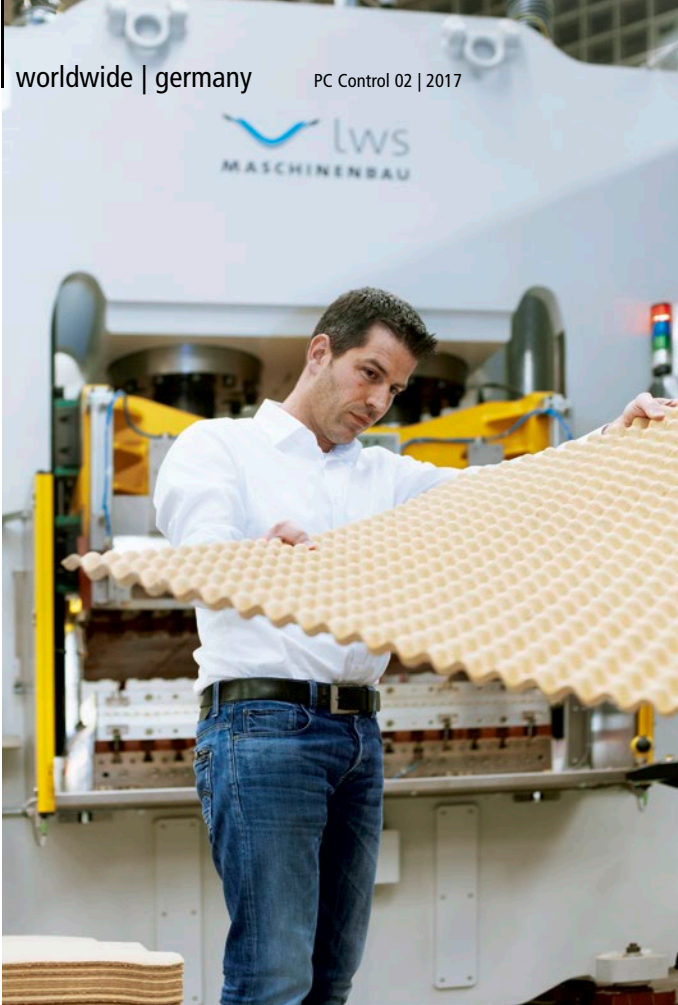
Michael Schäpers, Managing Partner of Lightweight Solutions, inspects the core structure of the Lisocore® lightweight construction material before it enters the hydraulic press.
