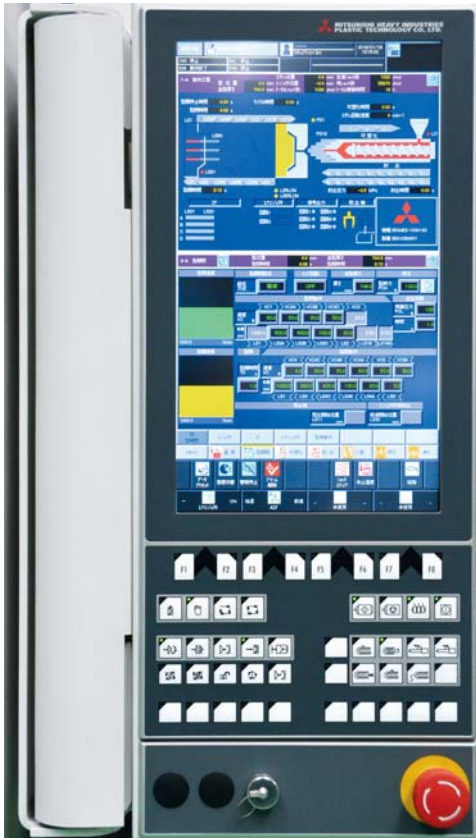
The MEIII controller is a Beckhoff CP6216 Panel PC.
