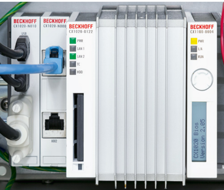
At the heart of the torque tester is a CX1020 Embedded PC which controls all test functions that are required for the qualification process.
