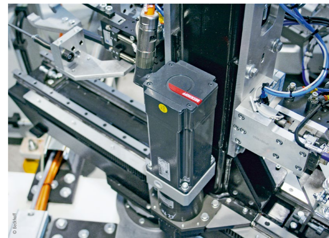
The distributed connection concept based on EtherCAT P and the compact AMP8000 servo drives save valuable space in the machine.
