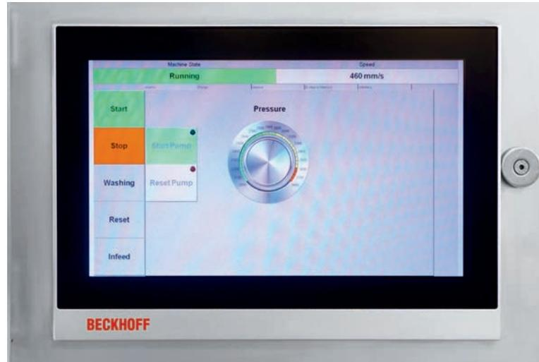
A customer-specific CP2911 Control Panel is used as HMI.
