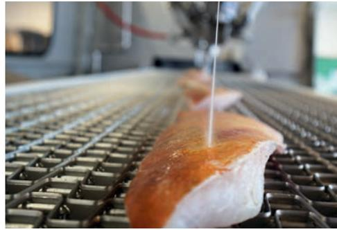
Cod fillets being portioned with water-jet cutting heads. The Valka cutter can process fish fillets at different cutting angles and remove bones with high precision.
