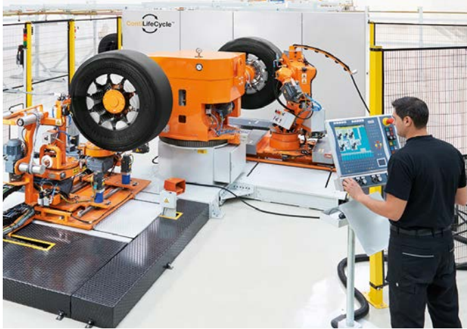
During the hot retreading process, an operator uses a Beckhoff CP7931 Control Panel with a 12-inch display, alphanumeric keyboard and add-on keys to apply a new rubber mixture to a truck tire's running surface and sidewalls.
