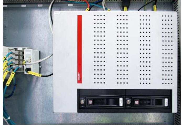
The C6650 control cabinet IPC provides ample performance to control even large multi-axis machines.
