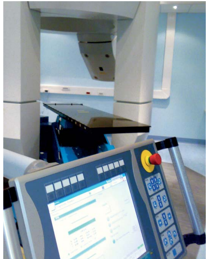
Beckhoff CP7911 Control Panel with emergency stop button and customized keypad
