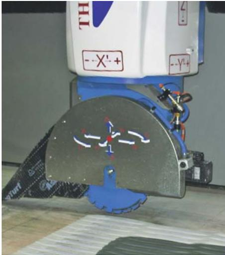
The T508 texture processing center from Thibaut handles polishing, matt grinding, antique brushing, gloss finishing and bush hammering of granite and other stone surfaces for interior decoration.
