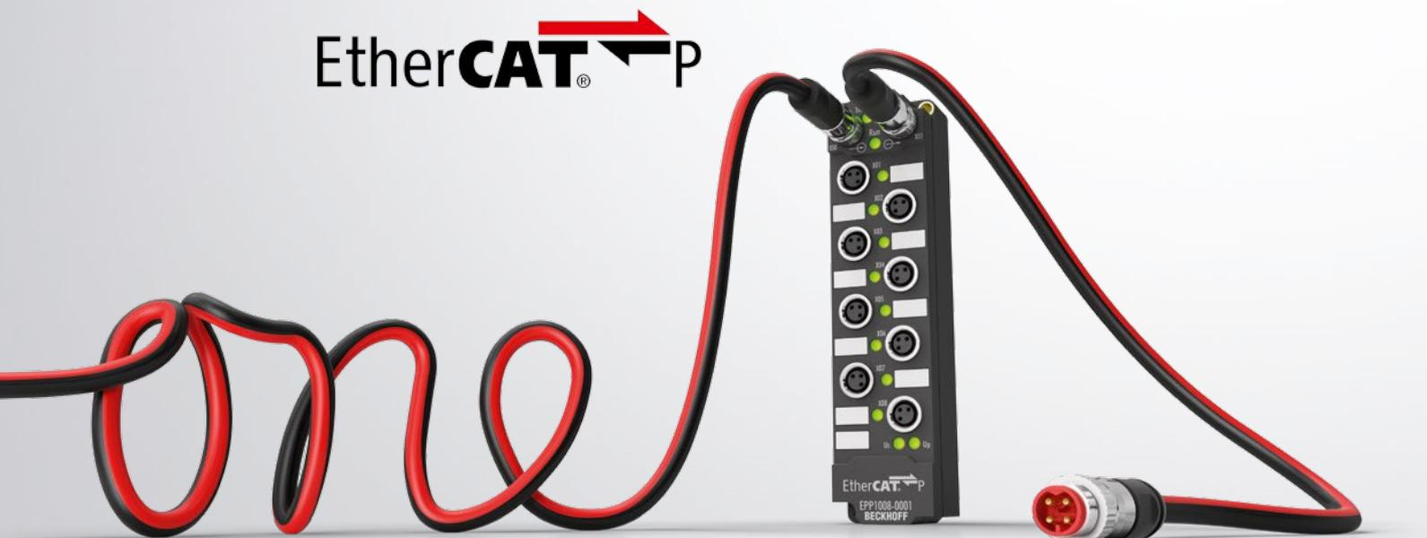
EtherCAT P combines the 24 V DC power supply for EtherCAT P slaves and connected sensors and actuators in a single 4-wire standard Ethernet cable.  $U_S$  (system and sensor supply voltage) and  $U_P$  (peripheral voltage for actuators) are electrically isolated from each other and can supply current of up to 3 A to the connected components.
