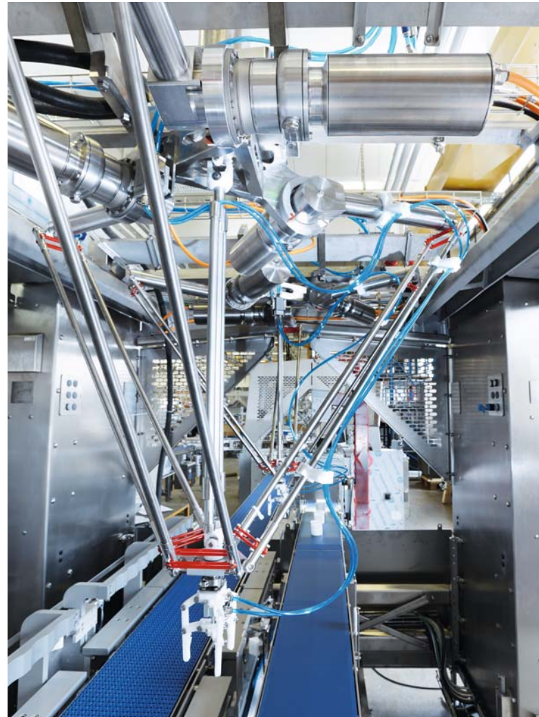
The AM8800 stainless steel motors can be used in open designs, i.e. without protective housings, facilitating optimal cleaning of pick-and-place robots.
