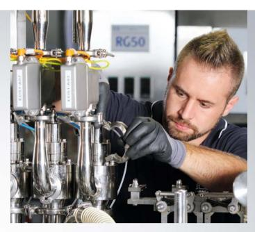
An intelligent metering system with a flow meter makes it possible to package liquids like milk or fruit juice, while a piston-based high-viscosity metering system is available for semi-liquid products like yogurt.
