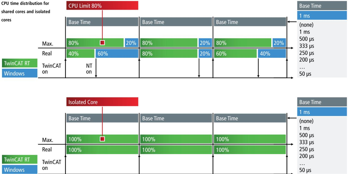
With the double tick, the computing time on a single processor core can be divided in such a way that timing functions necessary for Windows are retained and Windows cannot be “stalled” by an excessively high real-time load. For example, Windows communication via a serial interface works perfectly even with higher baud rates, which would not be possible without the double tick.
