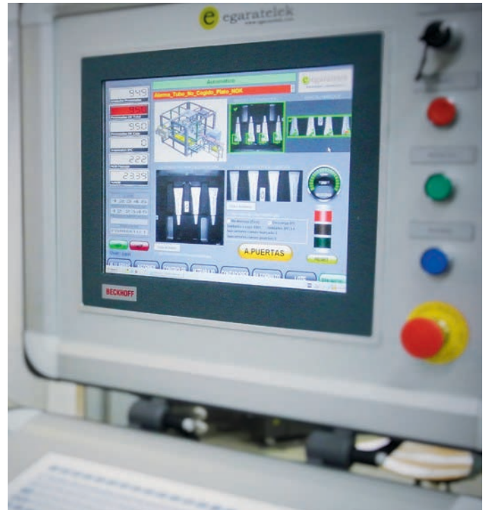
A CP6202 Panel PC is used as HMI for the laser marking machine.
