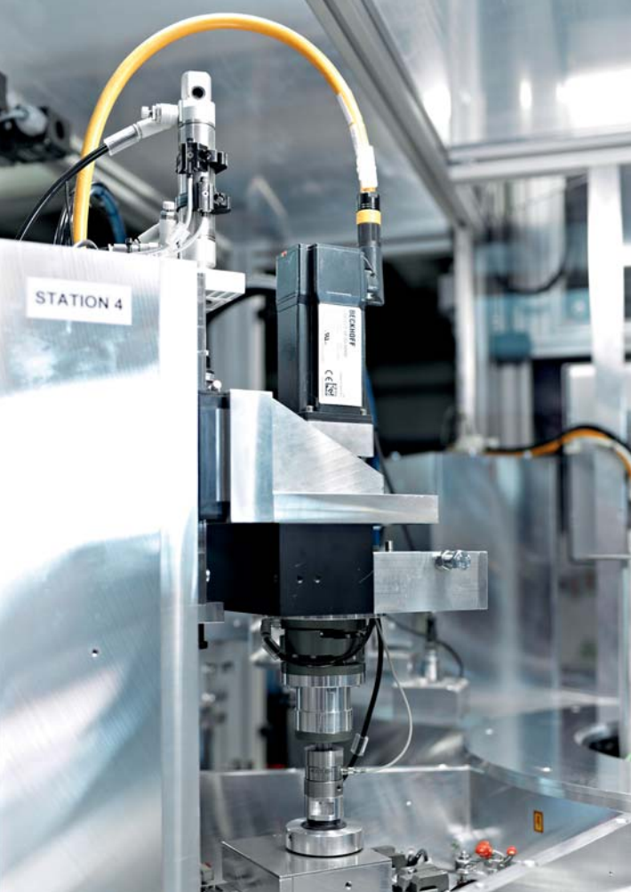
The AM81xx OCT servomotors ensure high-precision movements in no less than seven axes.
