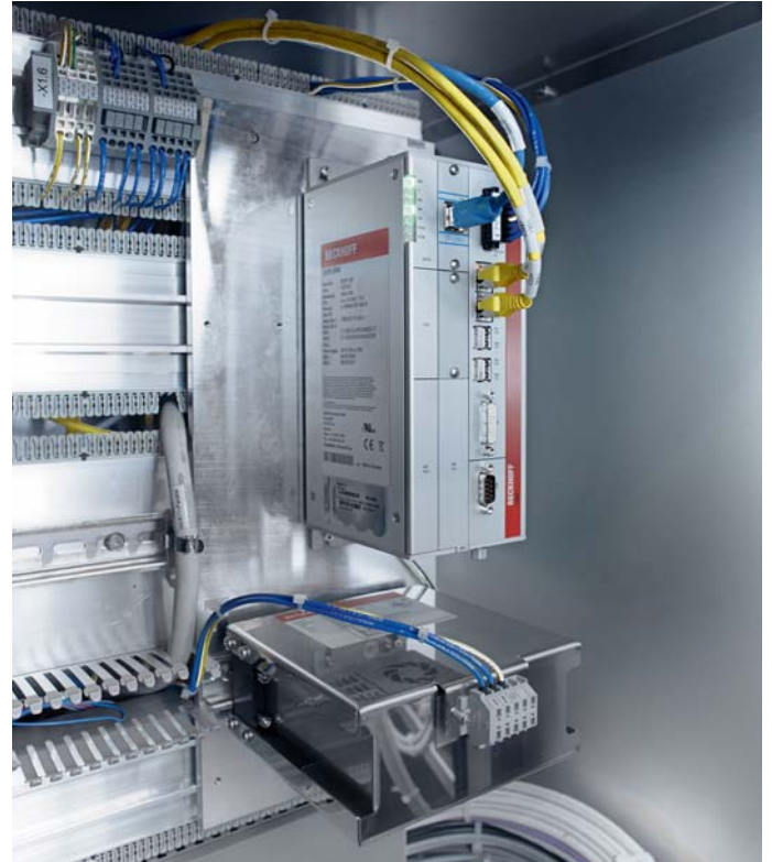
The C6930 control cabinet IPC – with Intel® Core™ i5 processor, SSD, and integrated UPS with additional 24 V battery pack – is connected to the operating panel via CP-Link 4.
