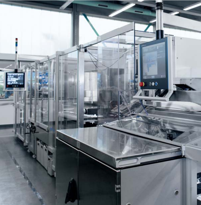
Two of the new operating units are used in the 10-meter long, two-track Blister Express Center BEC 500.
