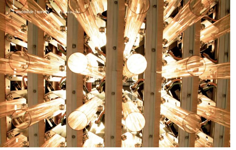
A total of 529 AM8121 servomotors and 529 EL7201 servo terminals were installed in order to move all the Plexiglas tubes.
