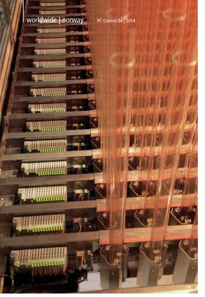
The compact electronics that control the 529 plexiglas tubes are installed at both ends of the support structure. The controls consist of an EK1100 EtherCAT Coupler, digital input terminals, servo terminals, and buffer capacitor terminals.
