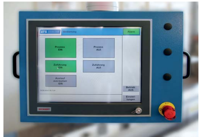
The 19-inch touchscreen on the CP6203 built-in Panel PC offers sufficient space for a clear display of the visualization created with TwinCAT HMI software.
