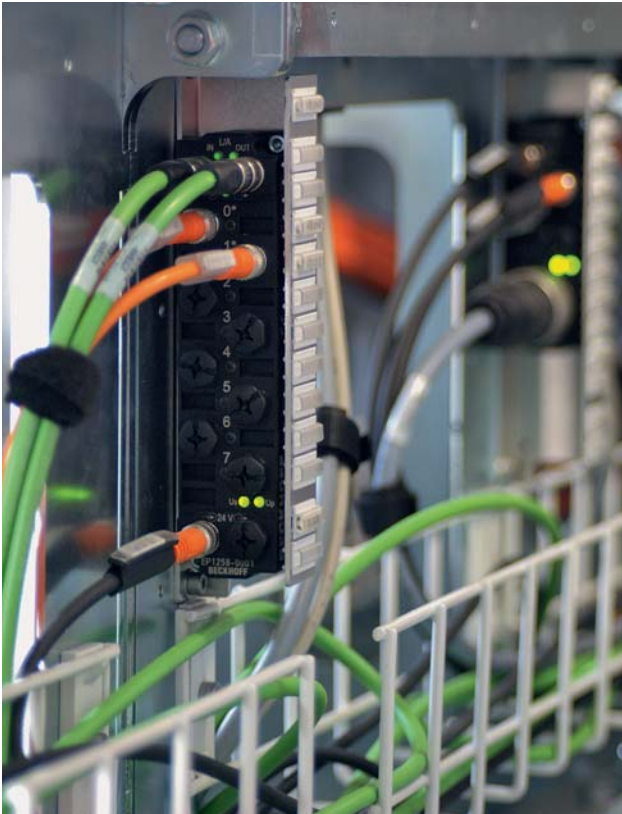
The workpiece carriers are identified as they drive past with the help of the digital EP1258 EtherCAT Box. Up to 623 different part carriers can be detected on the transport system.
