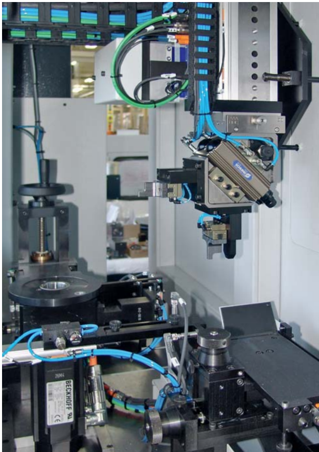
3-axis handling device for the grinding machine
