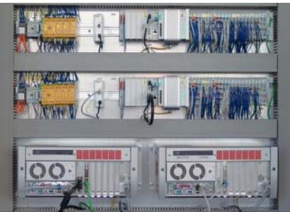
Control cabinet for controlling at rotary dial and index machine with 12 positions. One C6240 Industrial PC is used for data acquisition and communication with the higher-level EDP system. A second C6240 deals with calculating the complex algorithms on the systems. Two CX1030 Embedded PCs with EtherCAT Terminals act as machine controllers.
