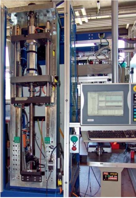
The hydraulic high-performance press (8 t), one of LCA's standard products, is controlled with TwinCAT.
