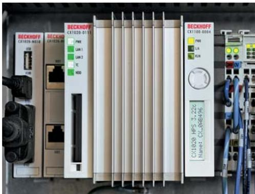
Beckhoff CX1020 Embedded PCs with the TwinCAT PLC automation software and EtherCAT I/Os are used as the control platform for the check weighers from Friesen's.
