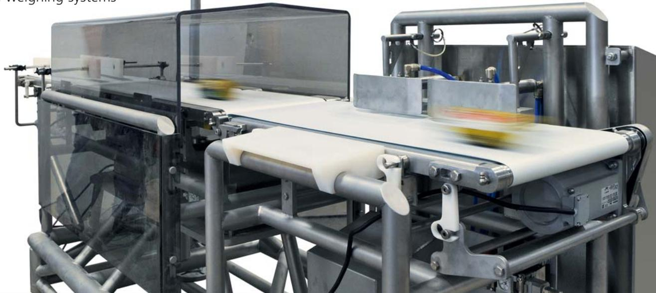
The American company Friesen's supplies material handling systems for the food industry, with particular focus on meat processing applications. By using open PC- and EtherCAT-based Beckhoff controllers in their weighing systems Friesen's was able to increase the process speed significantly while at the same time offering high precision.
