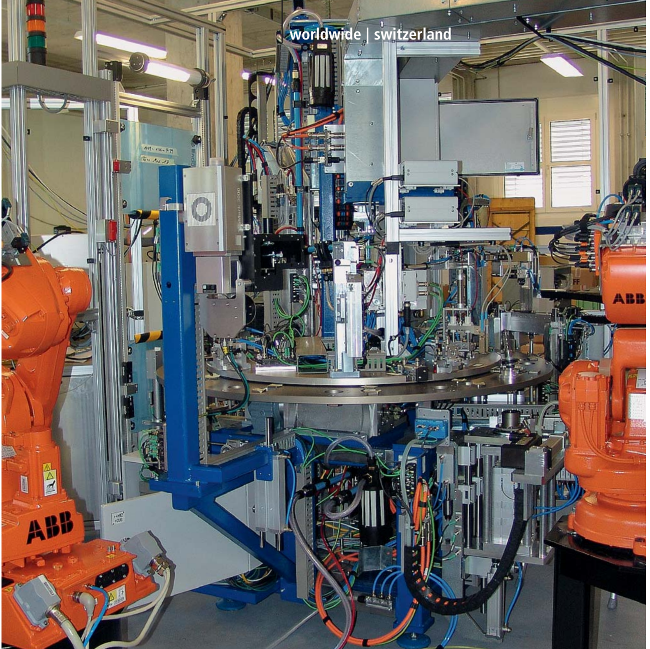
Rotary dial and index machine with 12 positions for complex processes with short cycle times. Two robots from ABB deal with inserting the blanks and removing the finished shafts.
