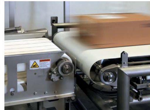
Through the application of PC- and EtherCAT-based controllers, Friesen's was able to reduce check weigher downtime by 22 % while increasing process speed by 31 %.
