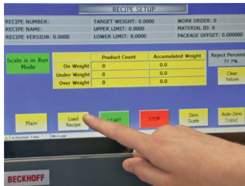
The weighing systems are visualized using a Beckhoff CP6902 Control Panel with 15-inch touchscreen.
