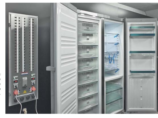
Fridge/freezer undergoing testing in the climatic chamber. To ensure that the appliances can be used worldwide, they are specified by 'climate categories,' and Miele checks in conformance with standards that category conditions are maintained.
