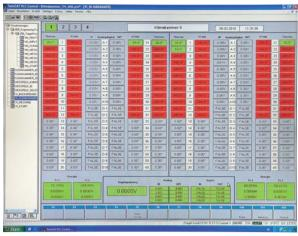
The stated aim is the highly accurate measurement and control of the temperature in the appliances and climatic chambers during the entire test period.
