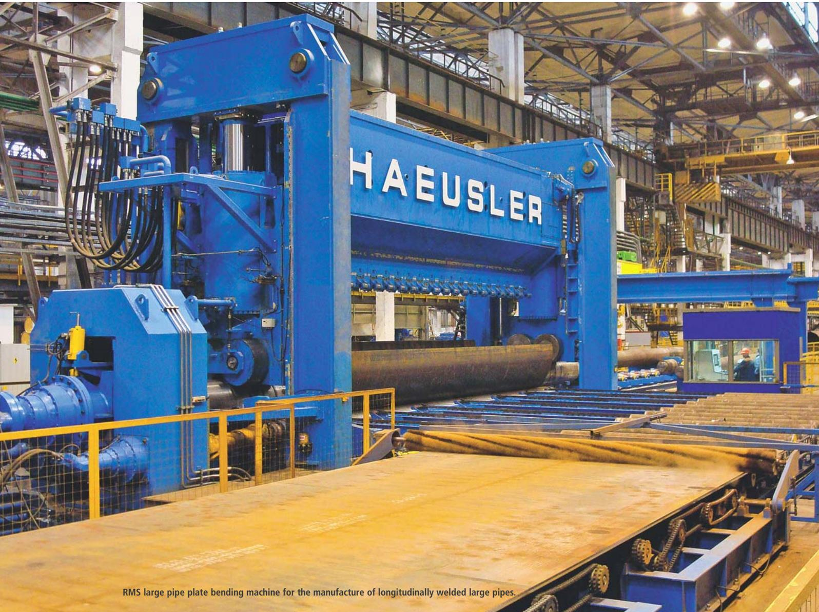
RMS large pipe plate bending machine for the manufacture of longitudinally welded large pipes.
