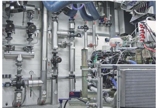
The heating and cooling circuits with pumps for the media conditioning
