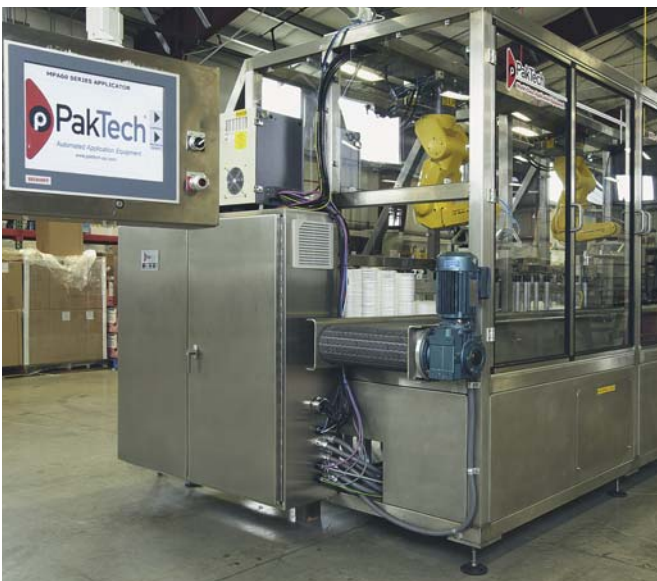
PakTech handle applicator for applying multi-pack handles on various bottles and packages
