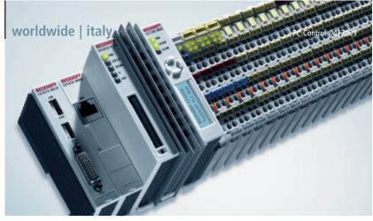
The Beckhoff CX1010 Embedded PC is used at CS Vacuum for controlling both production and the complex airconditioning system.
