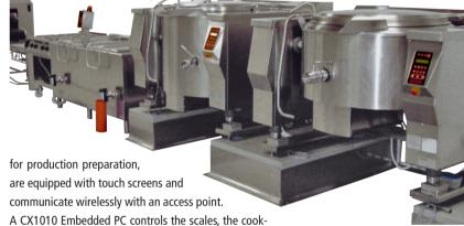
ing pot and the fryer (via Modbus) as well as the oven (via PROFIBUS).
