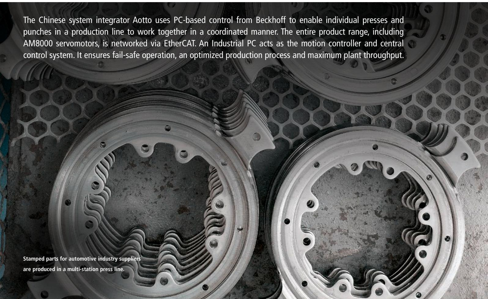
Stamped parts for automotive industry suppliers are produced in a multi-station press line.
