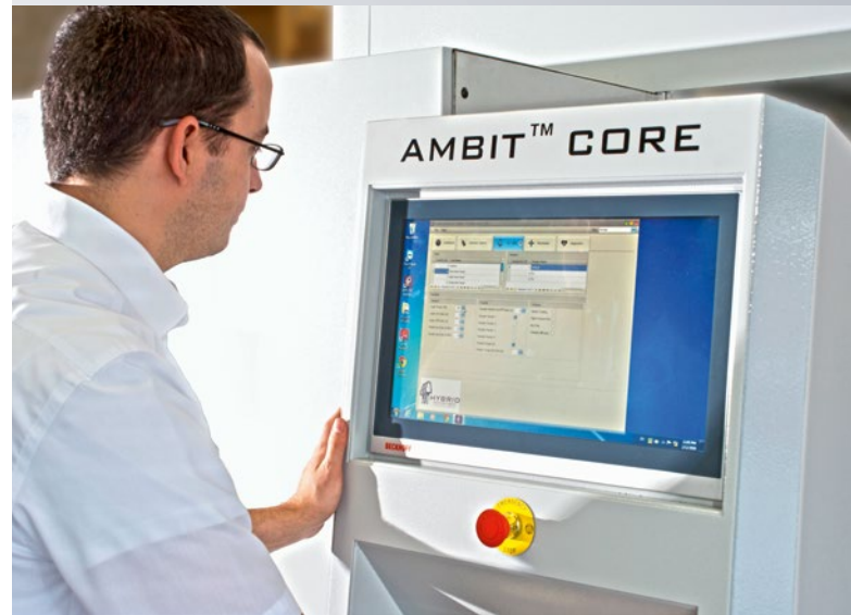
The hybrid system is controlled via a Beckhoff CP2218 multi-touch Panel PC.
