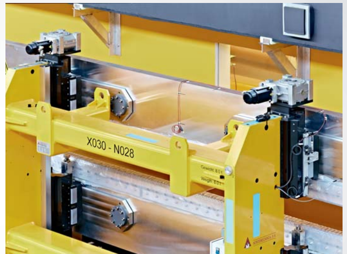
A total of four AM3052 servomotors per undulator cell – controlled via TwinCAT NC PTP – ensure that the magnet structures are precisely positioned. (The image shows the two motors of the upper magnet structure)
