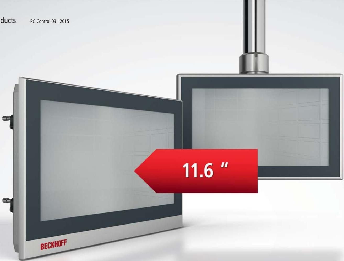
High degree of scalability, with nine display sizes for Panel PCs and Control Panels
