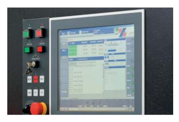
The Beckhoff CP6902 built-in Control Panel with touch screen provides convenient operation and monitoring of the turret punch press.
