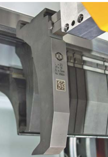
A scanner recognizes the tools and inserts them with pinpoint accuracy into the cheeks by means of a matrix code.
