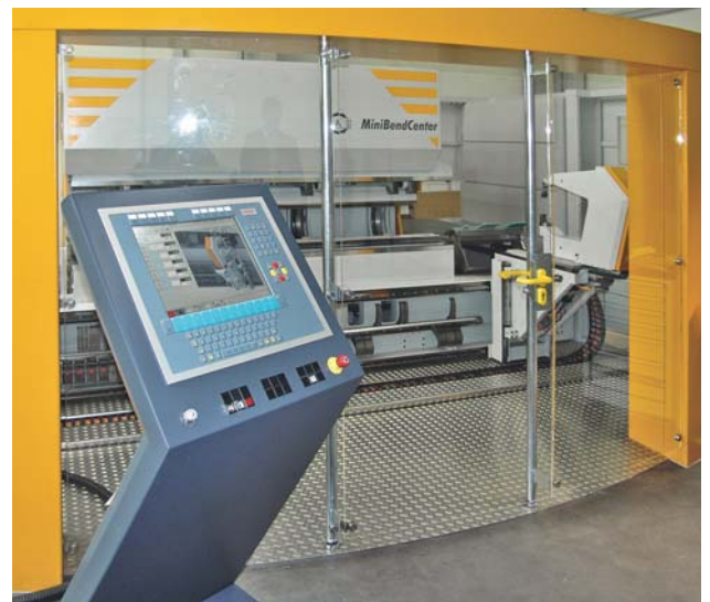
A Control Panel detached from the Industrial PC serves as an operating and visualization platform.
