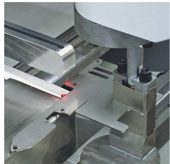
Once three points of the blank have been measured, the system knows the precise take-up position of the blank and corrects all deviations from the theoretical gripping position of the manipulator on the way to the first bending station.
