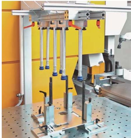
A suction system grips the uppermost blank and brings it to the transfer table, where a manipulator takes over the part. This guides the sheet past an optical measuring station in the first step.
