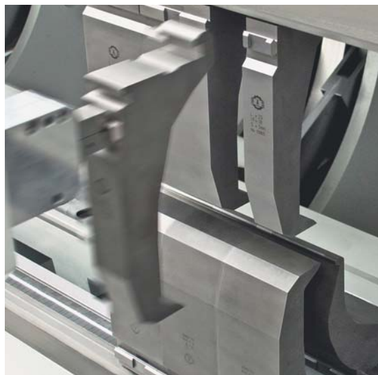
Before bending begins, a tool changer equips the individual bending stations automatically. The machine controller receives the necessary tool lengths per station from the CAM system.
