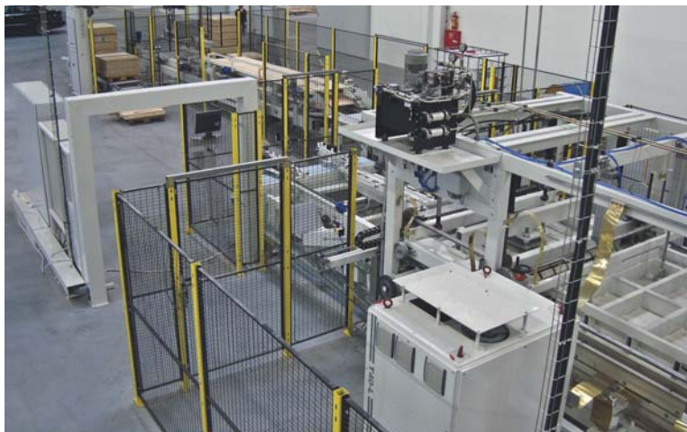
Continuous press line for the non-stop gluing, pressing and cutting of the glued boards for the furniture industry. The machine is 41.2 m (135.2-ft) long and consists of a portal in-feeder, sorting line, gluing station, continuous high-frequency press, board-trimming saw and palletizing station.
